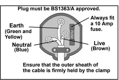
We strongly recommend that this machine is connected to the mains supply through a Residual Current Device (RCD)
